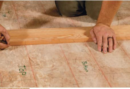
A critical step. After numbering each board's position on the grid, check the accuracy of the marks against those on the floor, and assign the orientation of each dado—whether it will face up or down. Once the horizontals have been marked, check the vertical boards and mark them in the opposite orientation.
