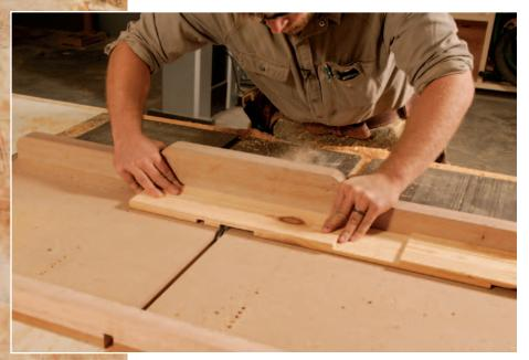
**Cut the dadoes.** The author milled the half-lap dadoes with a dado stack and a 4-ft.-wide crosscut sled, making sure to have plenty of room and support for the boards on either side. Each dado's orientation was marked on the edges, so he flipped the board back and forth as he went. It's easier to cut to the lines on either side of the dado and then to plow the remainder away.
