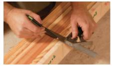
Gang layout. The pole comes back into play for marking the flooring stock for dadoes. Clamp all the boards of the same orientation to the story pole, and use a combo square to mark off the layout.
